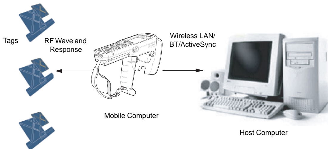
Figure 1-1 RFID System Elements
