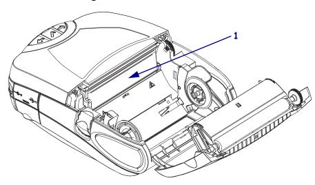
Figure 6 • RP4T Antenna Location
